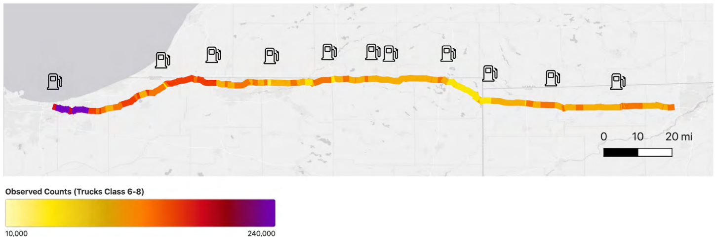
Fig. 2 – Class 6, 7 and 8 diesel truck volumes along the I-80/I-90 corridor between Chicago and Toledo, with diesel refuel site locations marked. All counts represent observed commercial vehicles.
